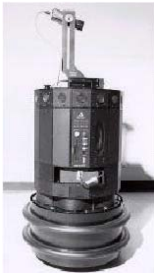
Figure 6. The Nomad 200 is a mobile robot equipped with a ring of 16 sonar sensors.
