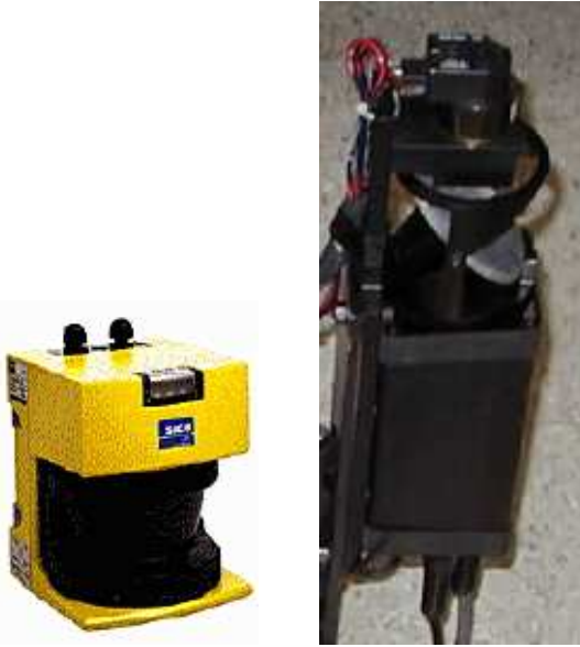
Figure 2: The SICK and AccuRange laser scanners. The SICK has a range of about 50 meters, coverage of 180 degrees, with a resolution of \pm 50 mm. The AccuRange 4000 laser has a range of about 25 meters, coverage of 360 degrees (minus the support structure for the mirror), and a resolution of \pm 50 mm.
